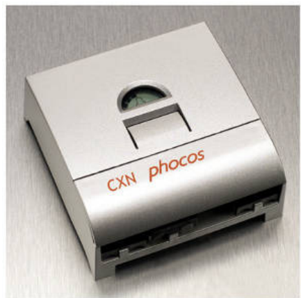
Rys. 4. Regulator ładowania CXN10-1.1 phocos, Programmable Solar Charge Controller with Negative Ground, 12/24V, 10/10A
